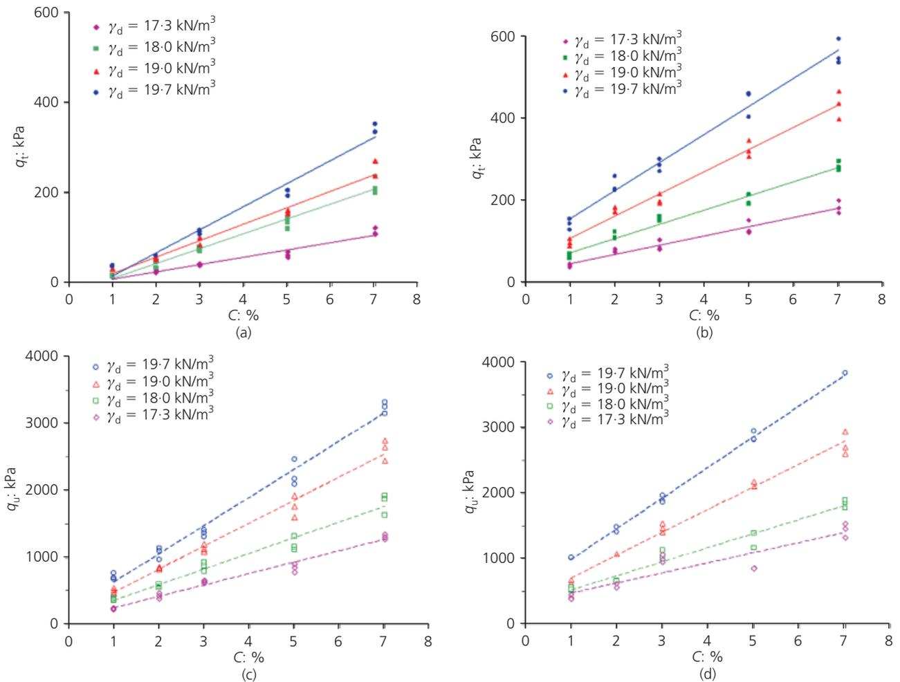
**Figure 2.** Variation of splitting tensile strength with cement content for (a) non-reinforced specimens and (b) fibre-reinforced specimens; and unconfined compression strength with cement content for (c) non-reinforced specimens and (d) fibre-reinforced specimens
