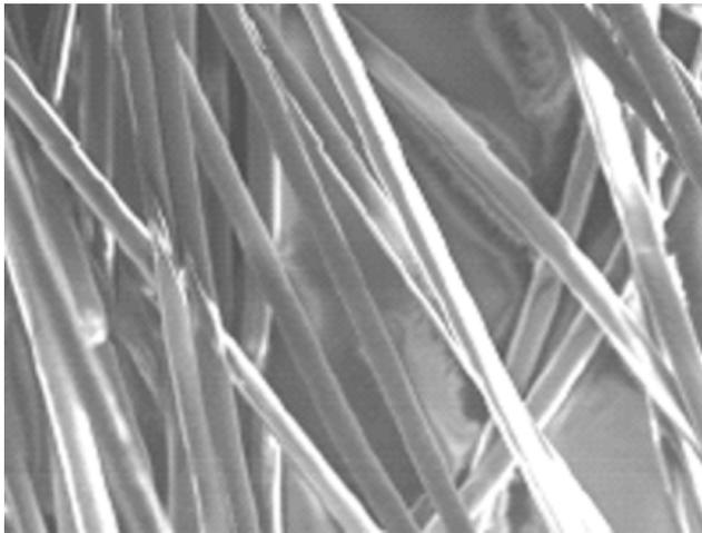
**Figure 1.** Picture of polypropylene fibres employed in present research
