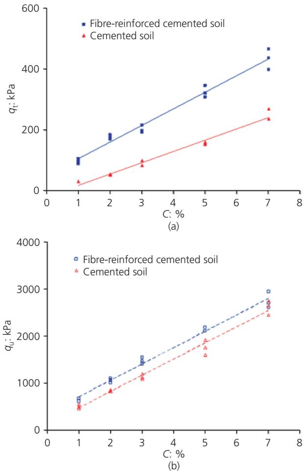
**Figure 3.** Variation of (a) splitting tensile strength with cement content for fibre-reinforced and non-reinforced specimens considering  $\gamma_d = 19.0 \text{ kN/m}^3$  and (b) unconfined compressive strength with cement content for fibre-reinforced and non-reinforced specimens considering  $\gamma_d = 19.0 \text{ kN/m}^3$
