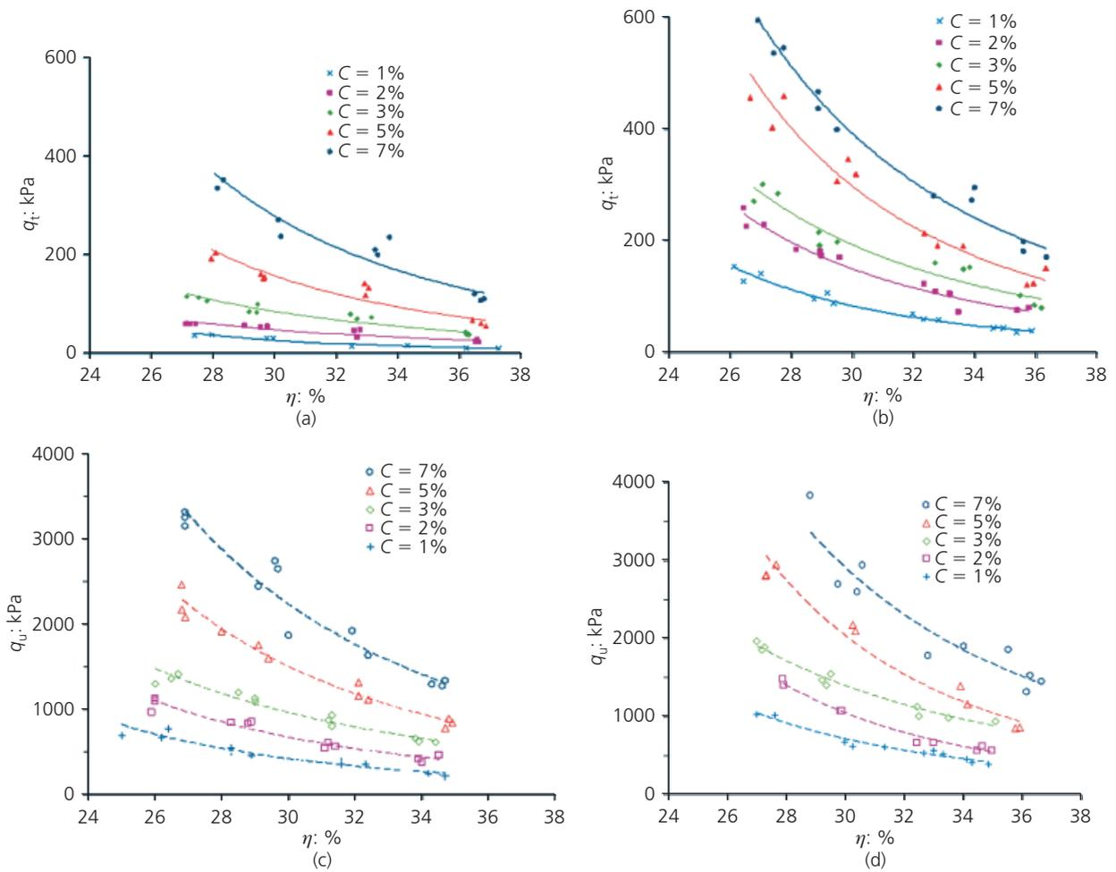
**Figure 4.** Variation of splitting tensile strength with porosity for (a) non-reinforced specimens and (b) fibre-reinforced specimens and unconfined compression strength with cement content for (c) non-reinforced specimens and (d) fibre-reinforced specimens
