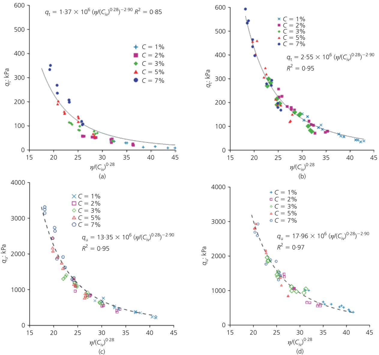
Figure 7. Variation of splitting tensile strength with adjusted  $\eta/C_{iv}$  for (a) non-reinforced specimens and (b) fibre-reinforced specimens and unconfined compression strength with adjusted  $\eta/C_{iv}$  for (c) non-reinforced specimens and (d) fibre-reinforced specimens
