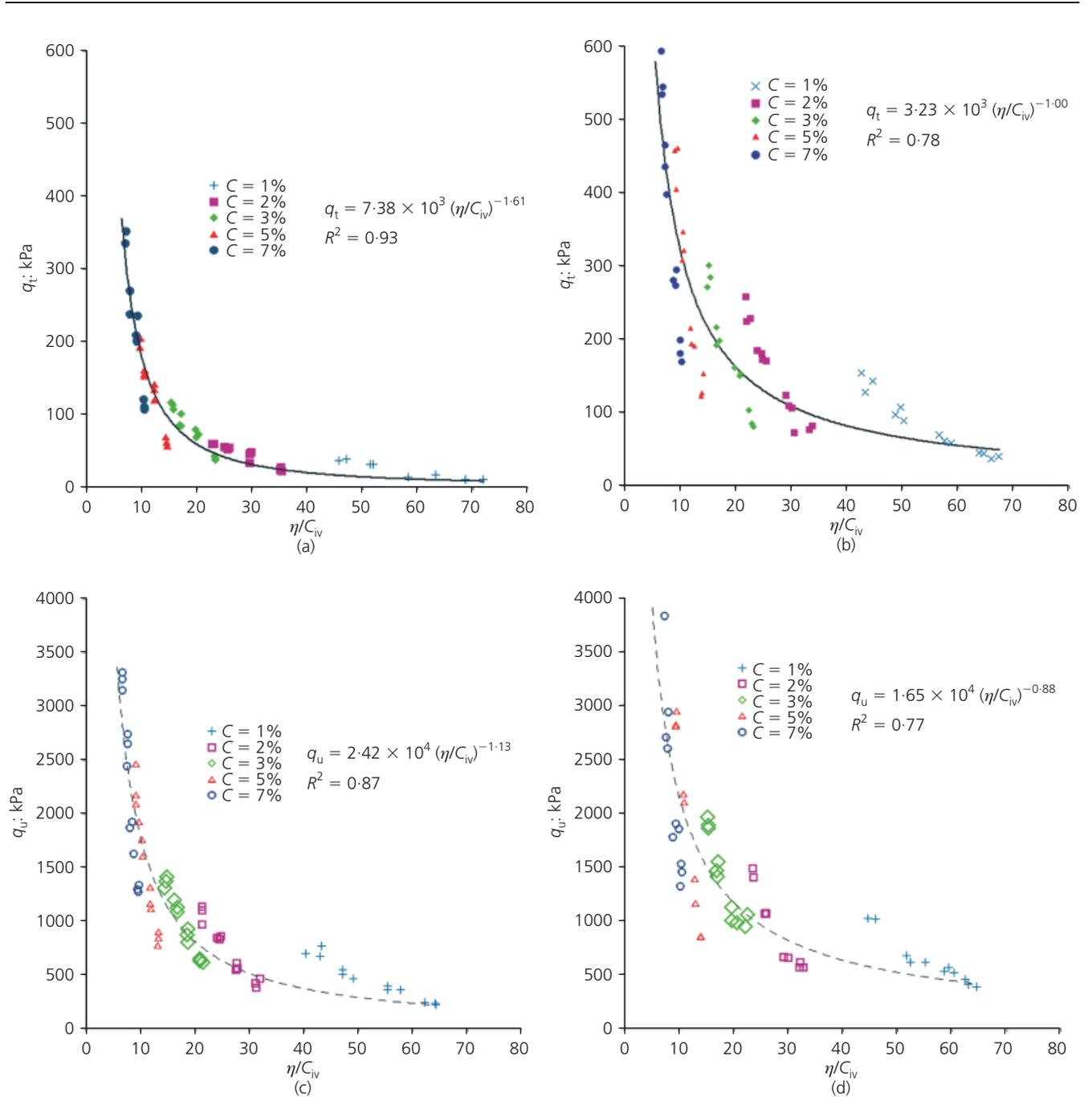
**Figure 6.** Variation of splitting tensile strength with  $\eta/C_{iv}$  for (a) non-reinforced specimens and (b) fibre-reinforced specimens and unconfined compression strength with  $\eta/C_{iv}$  for (c) non-reinforced specimens and (d) fibre-reinforced specimens
