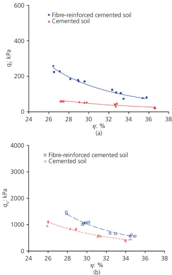
**Figure 5.** Variation of splitting tensile strength with porosity (a) for fibre-reinforced and non-reinforced specimens considering  $C = 2\%$  and (b) unconfined compressive strength with porosity for fibre-reinforced and non-reinforced specimens considering  $C = 2\%$
