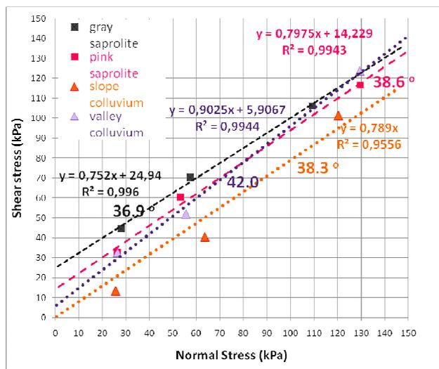
Figure 5 Shear strength envelope for the 04 soils studied.
