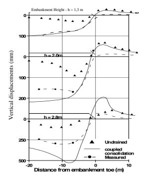
**FIGURE 2.** Settlements at the embankment I base at various stages of construction.
