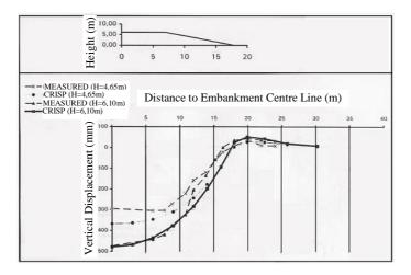
**FIGURE 3.** Computed and measured vertical displacements at the base of the Juturnaíba embankment (Antunes, 1996).
