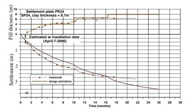
**FIGURE 5.** *Typical settlement plate data of Recreio embankment (Almeida et al., 2008).*
