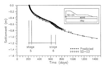
**FIGURE 4.** Predicted and measured settlements at Sergipe breakwater (Brugger et al., 1998).
