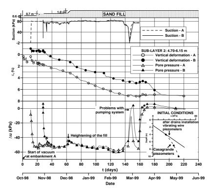
**FIGURE 10.** Vertical deformation of sub-layers 2A and 2B (fill B) and pore pressure measured in the middle of these layers, at a depth of 5.4 m (Marques and Leroueil, 2005).
