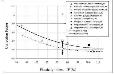
FIGURE 1. Vane strength correction versus plasticity index Brazilian case
