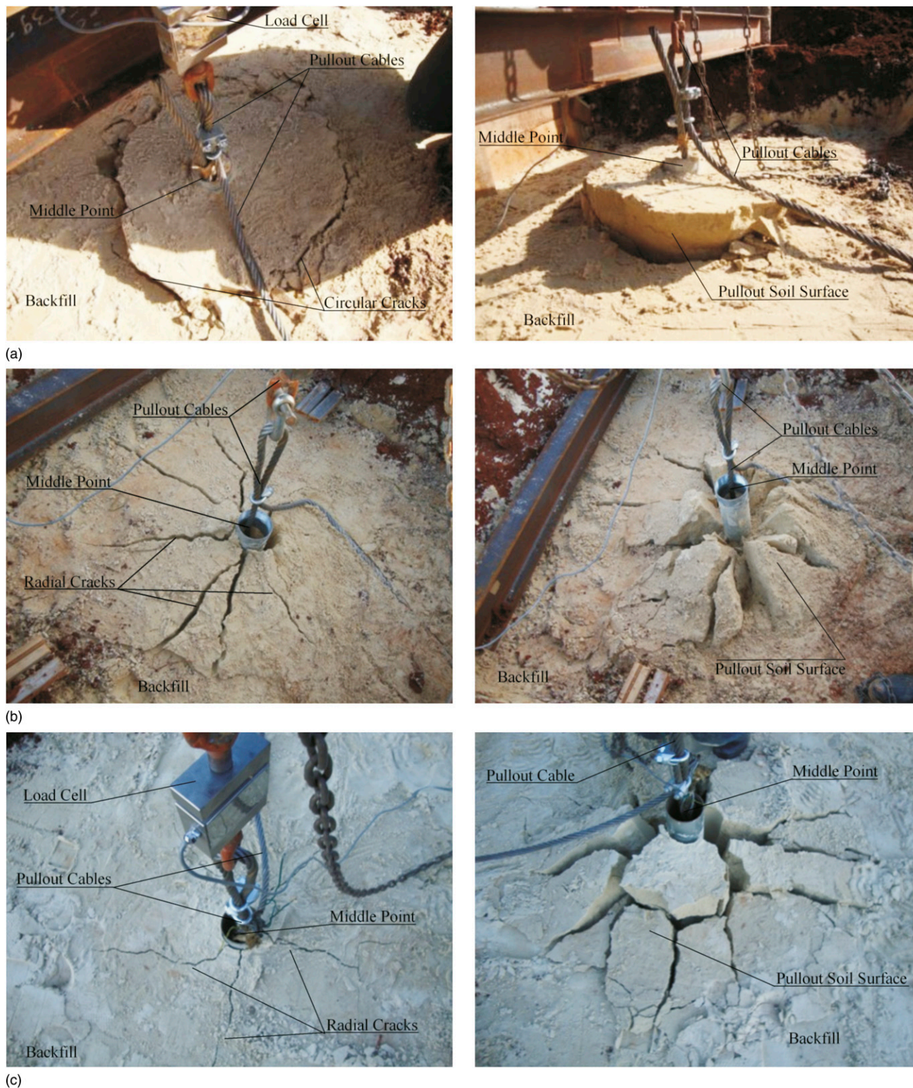
Fig. 6. Photos of the pullout failure mechanisms in sand layers considering anchor plates with distinct normalized embedment depth (a) H/D = 1.0 , (b) H/D = 1.5 , and (c) H/D = 2.0
