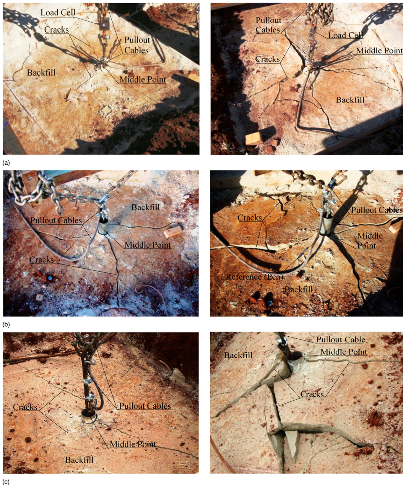
Fig. 7. Photos of the pullout failure mechanisms in sand-cement layers considering anchor plates with distinct normalized embedment depth (a) H/D = 1.0 , (b) H/D = 1.5 , and (c) H/D = 2.0
